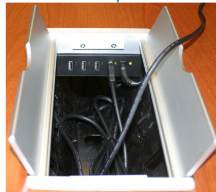
USB inputs for mice, keyboards, USB flash drives and a power strip.
